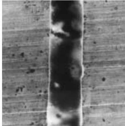
LaserScreen slot showing sharp slot edge and smooth working face (magnification x 260). 100 MICRONS: _____
